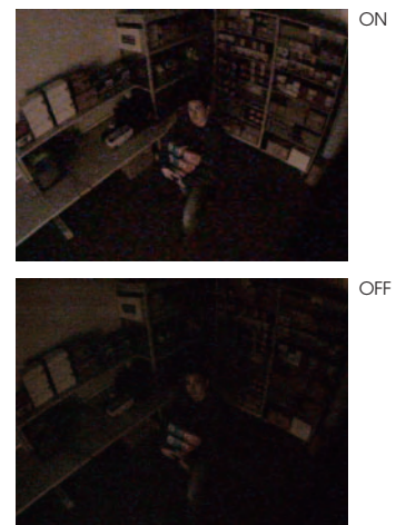
Fig. 3 (actual images) Light Funnel Function in 0.3 lx lighting conditions * When the light funnel function is activated, the image resolution is 640 x 480 (VGA).
